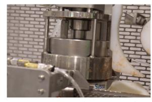
STEP 3: Automatically Opening the Cans with Crown Punch
