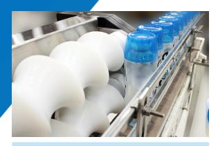
Our standard drive unit models include single, dual, or stacked screw systems to metering your containers for a variety of packaging applications.
